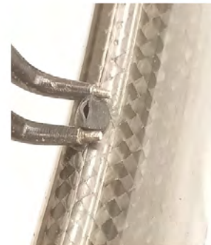
The silicone valve is slit to allow for the evacuation of internal air leaks.
